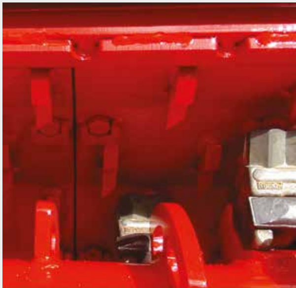
Grinding chamber fitted with counter knife shearbars
