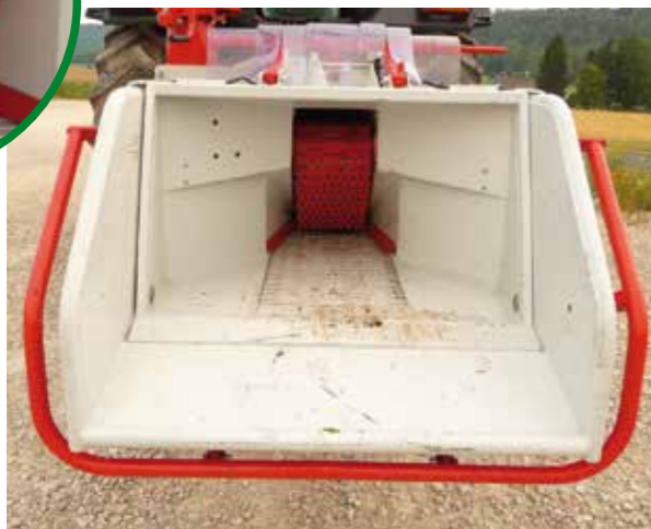
Upper intake feeder on all the models to ease to loading and lower intake conveyor as standard on the models CBB 300 and 300A (optional on the CBB 220 and 220A)
