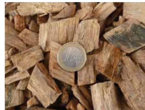
It is possible to ensure an even chip size thanks to the chip gauging grate.
