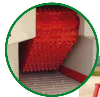
Upper intake feeder on all the models to ease to loading and lower intake conveyor as standard on the models CBB 300 and 300A (optional on the CBB 220 and 220A)
