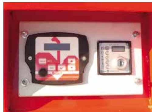
NO STRESS system, with 3 programs that control intake feeders speed
