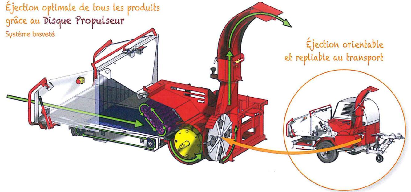
Éjection orientable et repliable au transport
