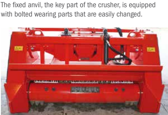
The high elastic limit steel rotor is machined from one piece of solid steel bar, and wearing parts are laid out in a spiral for uniform crushing.
