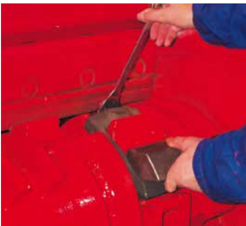
The QUICKCHANGE wearing part mounting system permits or wearing parts to be changed quickly. A locking system prevents the brackets from working loose.
