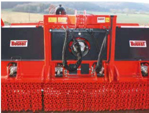
The anvils safety mechanism is controlled from the tractor seat thanks to a pressure gauge.
