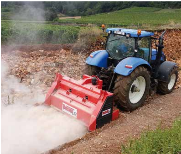
The anvils safety mechanism is controlled from the tractor seat thanks to a pressure gauge.
