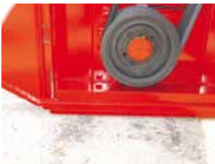
Several skids can be removed in order to enable the rotor level to be set below the skid level.
