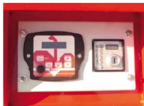
NO STRESS system, with 3 programs that control intake conveyor speed
