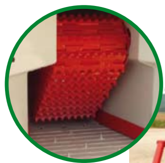
The upper intake conveyor eases loading on all models and a lower intake conveyor is standard on the CBB 300A (optional on the CBB 220A)
