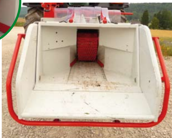
The upper intake conveyor eases loading on all models and a lower intake conveyor is standard on the CBB 300A (optional on the CBB 220A)
